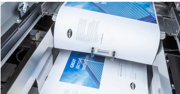
Collating station with the "tumbler" folding a sheet over to the station
