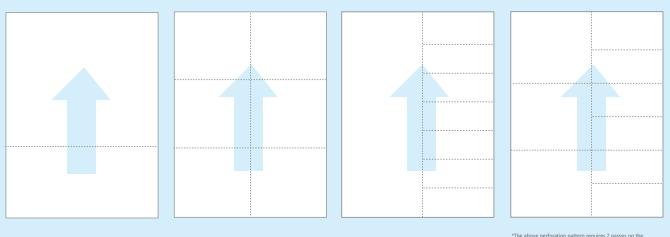
Examples of short edge fed perforating with optional perforation blade
