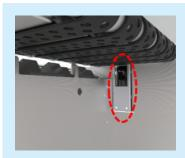
Morgana's Adaptive Process Control technology (APC) measures sheet separation in the "float area" and adjusts tray position and airflow automatically.
