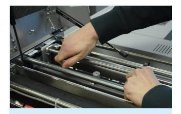
The Easyblade quick release mechanism enables changing crease blade for different jobs, without any special tools in less than 30 seconds. Extremely useful when changing between a perforation job and a creasing job.
