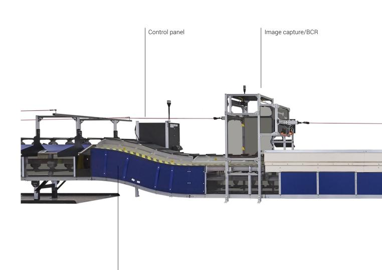
Incline - allows operators to be at ground level
