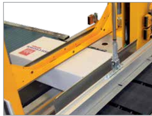
Package/Bundle stops to position loose bundles or packages
