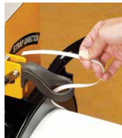
Simple coil change: Minimum downtime for coil change thanks to automatic strap threading
