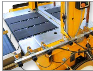
Photocell - Second strapping tension, package height control
